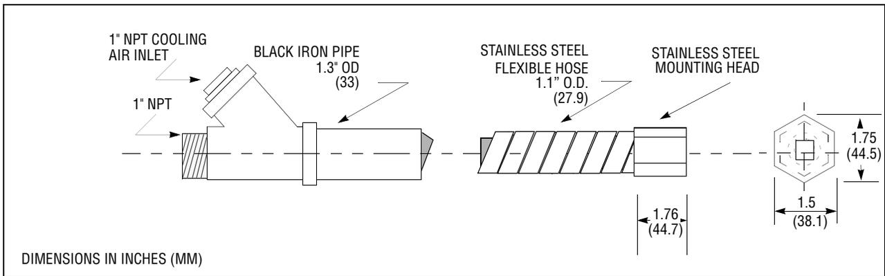
**FIGURE 3. INNER CARRIER ASSEMBLY**
