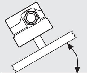
When installed in other position the pressure switch switches at pressure deviating from the set reference value by max.  $\pm 0.2$  in. W.C. (0.5 mbar).
