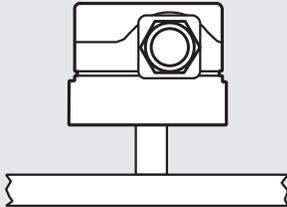
When installed horizontally, the pressure switch switches at a pressure higher by approximately 0.2 in. W.C. (0.5 mbar).
