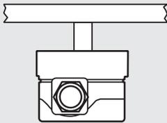
When installed upside down, the pressure switch switches at a pressure lower by approximately 0.2 in. W.C. (0.5 mbar).
