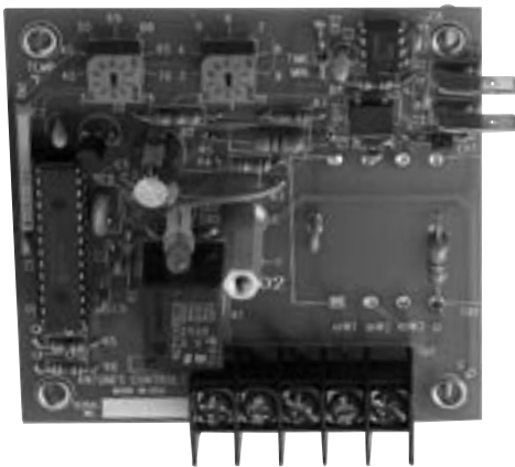
3" x 3" open board construction with stand offs. Optional cover is shown.
