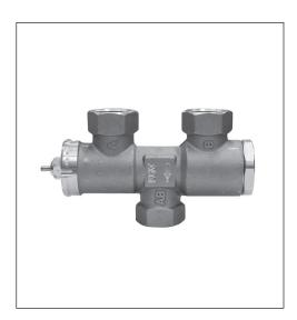
The Danfoss KOVM is a linear 3-way mixing valve with a unique bypass design allowing for constant system pressures and flow rates. When the KOVM is combined with either the RAVK non-electric thermostatic operator or the ABV 24VAC thermo-wax actuator the linear actuation of the valve results in the control of hot or chilled water flow to radiators, convectors, fan coil units, etc.
