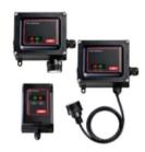
Utilizing either Semi-Conductor (SC) or Infrared (IR) technologies, DGS leak detectors give a rapid response when detecting a wide range of different refrigerants, including CO<sub>2</sub>. The DGS sensors can be used in stand-alone or integrated systems where continuous real-time, automatic monitoring is required. The DGS complies with environmental regulations and Health & Safety requirements on new or existing systems.
