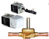
EVR and EVRH solenoid valves are direct or servo operated for liquid, suction and hot gas lines. They are available in both normally closed (NC) and normally open (NO) versions and feature interchangeable AC and DC coils. In standard applications standard BX/BJ coils are suitable to apply to EVR and EVRH valves; however, in applications with significant pressure differentials high MOPD BX/BJ coils are recommended. These can be found on page 10.
