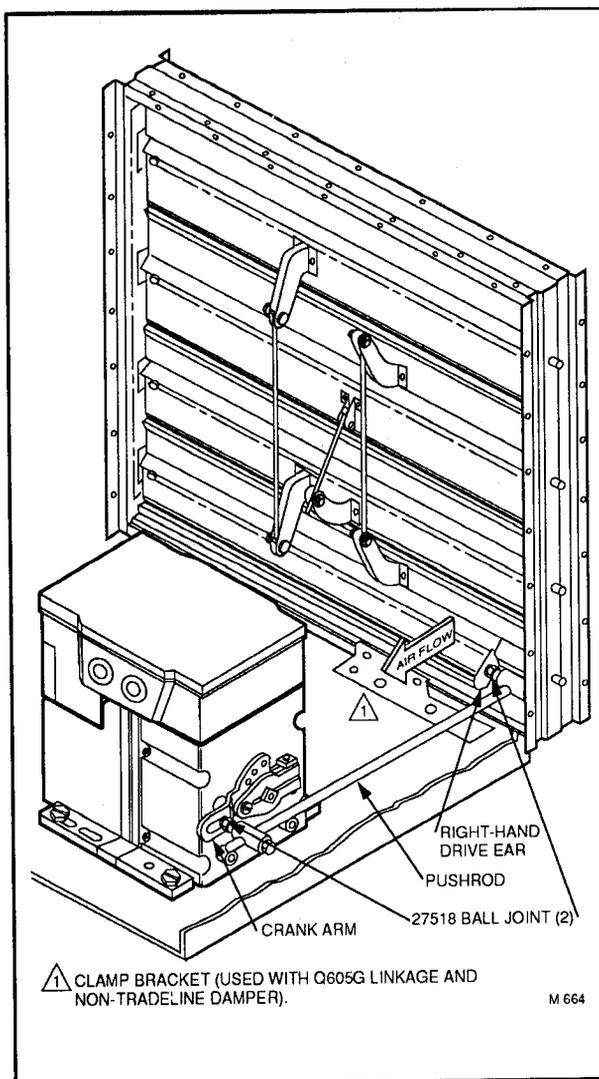
FIG. 8—MOUNTING MOTOR INTERNALLY WITH A HORIZONTAL DAMPER.
