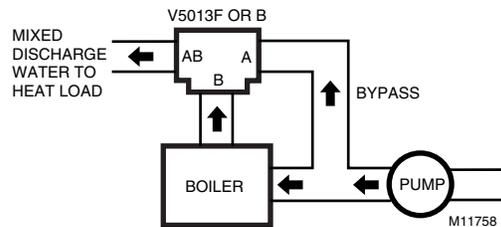
Fig. 5. Single zone bypass for reset control.
