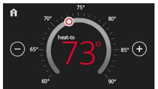
On the Home Screen, touching the heat setpoint indicators 0 on the round temperature band, or touching the heat-to button displays the heat menu screen.
