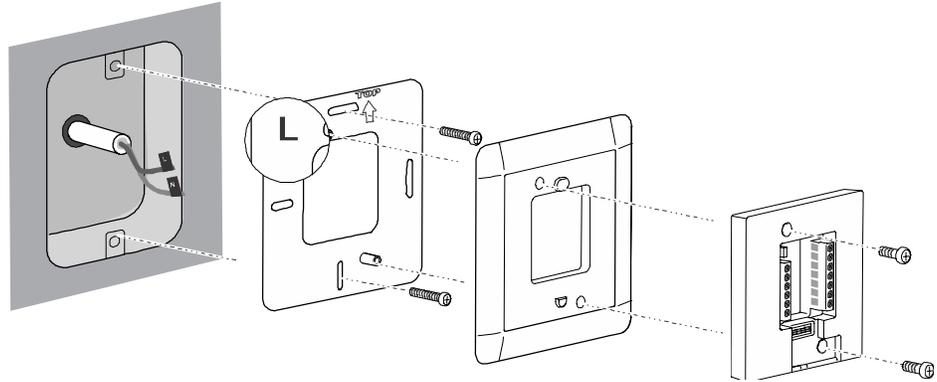
**Tip:** Before installing the power unit, it is highly recommended the labeled wires be connected to the terminals snugly according to the thermostat terminal designations (you may also refer to the picture taken in Step3). Do not overtighten.
