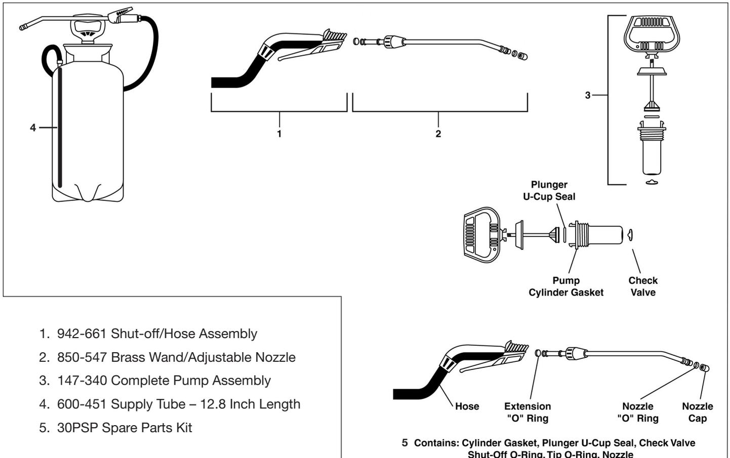
**IMPORTANT:** Replacement parts for No. 220CP Sprayers made AFTER June 2018, are blue inked sprayer tanks and are supported with parts used in other premium sprayers. No. 220CP Sprayers made before June 2018 use black inked sprayer tanks and require different replacement parts – contact Nu-Calgon.
