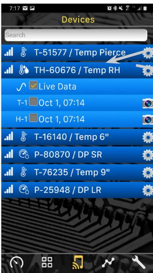
**Fig. 8:** Devices screen with live data selected.
