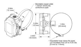
Fig. 3: Clamp-On Strap Unit in BAPI-Box (BB) Enclosure
