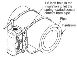
Fig. 7: Spring Loaded Strap Unit Mounting (BAPI-Box 2 Enclosure shown but mounting is similar for all BAPI-Boxes.)
