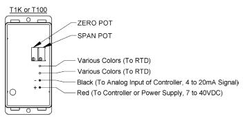
Fig. 8: Typical RTD 4 to 20 mA Transmitter with Flying Leads
