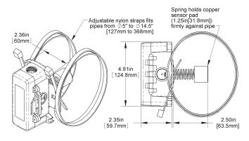
Fig. 5: Spring Loaded Strap Unit in a BAPI-Box 2 (BB2) Enclosure
