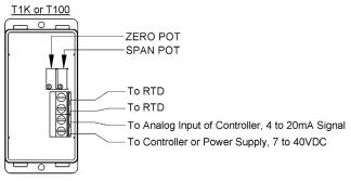
Fig. 9: Typical RTD 4 to 20mA Transmitter with Terminals
