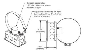
Fig. 1: Clamp-On Strap Unit with Junction Box (Standard)
