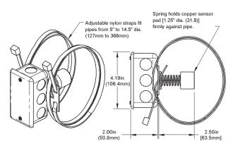
Fig. 4: Spring Loaded Strap Unit in a Junction Box (Standard)
