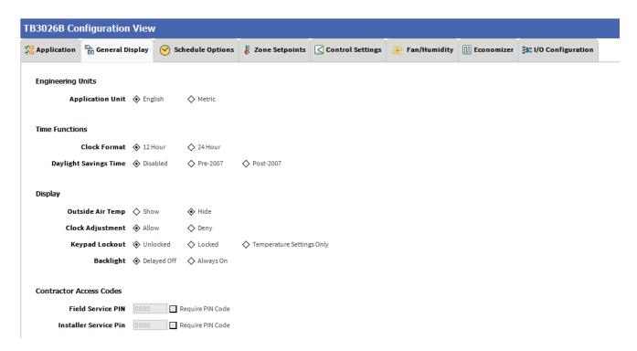
Figure 34: General Display Screen (AHU)
