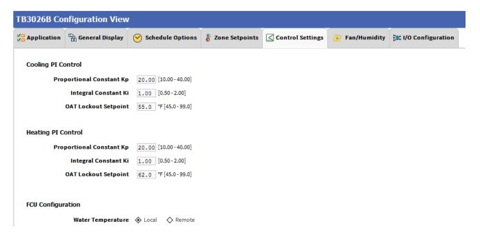
When 'Valve Actuator' is selected as 'Two-Position', the 'Control Settings' view changes as follows:
