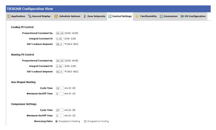
Figure 58: Control Settings Screen (Water Source Heat Pump)
