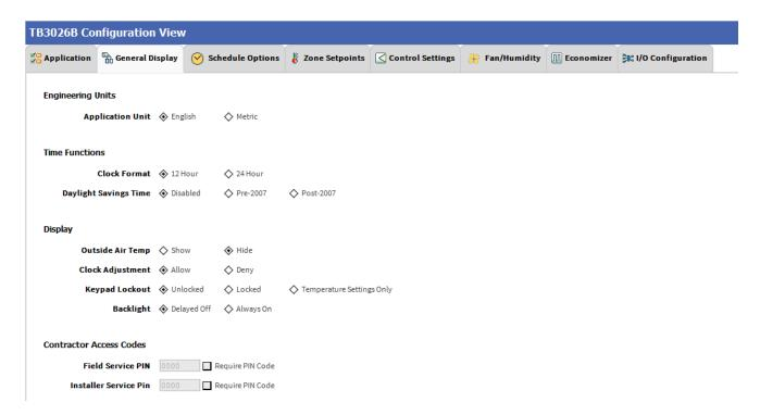
Figure 54: General Display Screen (Water Source Heat Pump)
