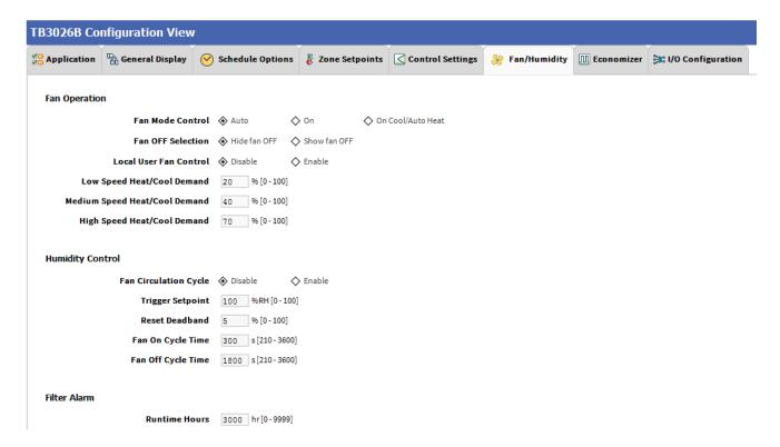
Figure 78: Fan/Humidity Screen (Four Pipe Fan Coil Unit)
