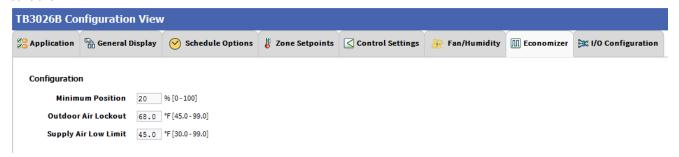
Figure 79: Economizer Screen (Four Pipe Fan Coil Unit)
