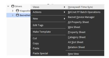
Figure 89: Selecting 'Honeywell Time Sync'
