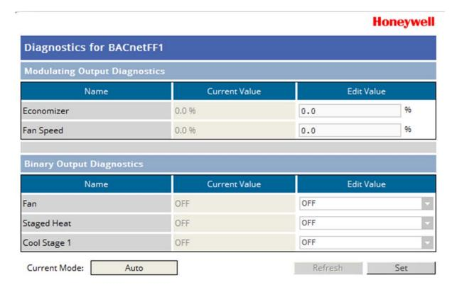
Figure 87: Outputs Overridden Mode/Diagnostics
