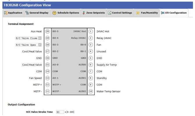
Figure 70: I/O Configurations Screen (Two Pipe Fan Coil Unit)
