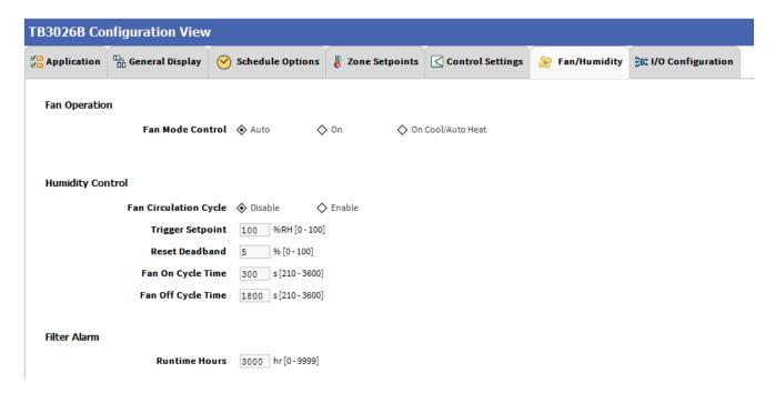
Figure 69: Fan/Humidity Screen (Two Pipe Fan Coil Unit)
