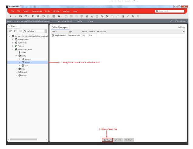
Figure 18: Adding BACnet Network
