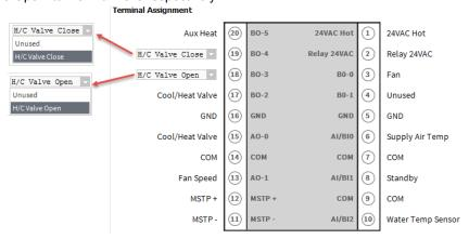
Figure 71: Terminal Assignment View (Single Speed Fan)
