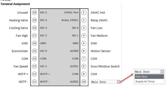
Figure 81: Terminal Assignment View (Three Speed Fan)
