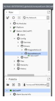
Figure 26: Drag and drop BACnetFF on BacnetNetwork
