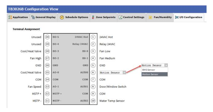
When 'Input Configuration is selected as 'Remote Space Temp Sensor' with 'No Stage Aux Heat', 'Floating/Analog' valve actuator and 'Three Speed Fan', the 'Terminal Assignment' view changes as follows:
