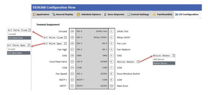
When 'No Stage Aux Heat' is configured with 'Two-Position' valve actuator, 'Three Speed Fan' and 'Water Temperature Sensor', the 'Terminal Assignment' view changes as follows:
