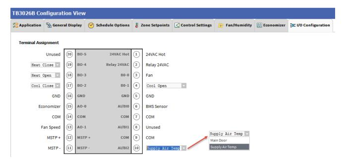
When 'Single Stage Aux Heat' is configured, the 'Terminal Assignment' view changes as follows:
