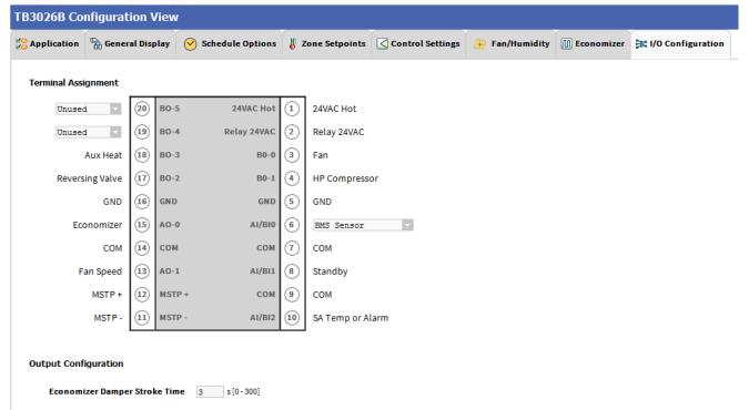
Figure 51: I/O Configurations Screen (Air Source Heat Pump)
