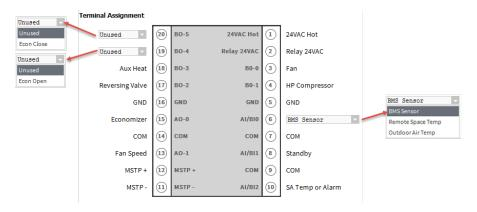
Figure 52: Terminal Assignment View (Air Source Heat Pump)
