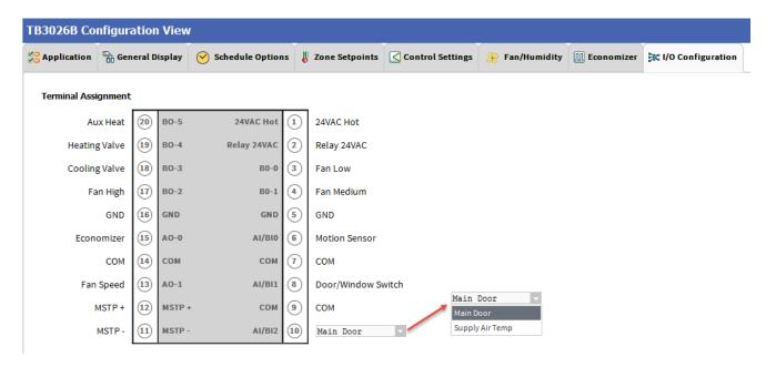
When Al/Bl2 is configured as 'Supply Air Temp' in (Application 9), Al/Bl1 gets displayed as 'Unused' and Al/Bl0 gets displayed as 'BMS Sensor' as follows:
