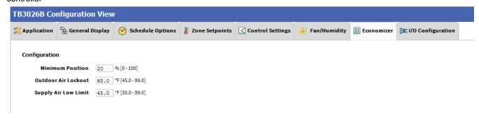
Figure 50: Economizer Screen (Air Source Heat Pump)
