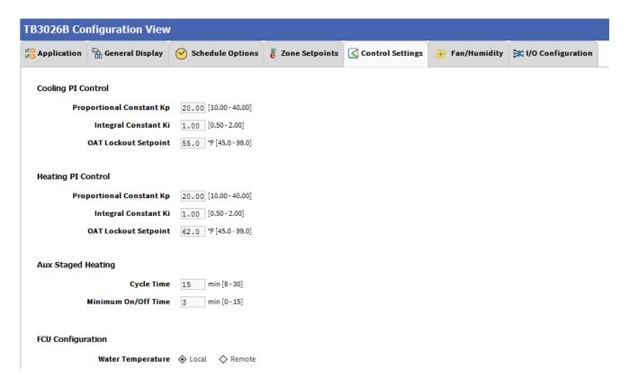
When 'Auxiliary Heat' is selected as 'No Stage Aux heat', the 'Control Settings' view changes as follows:
