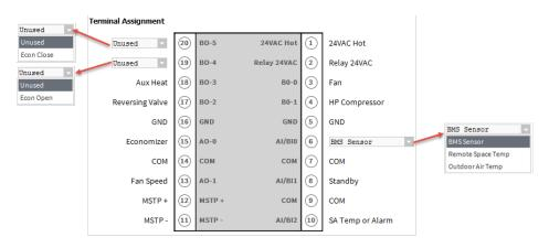
Figure 62: Terminal Assignment View (Water Source Heat Pump)
