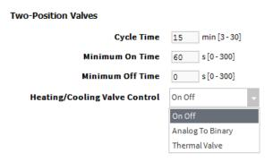
**Cycle Time:** Two-Position Valve cycle time ranges from minimum of 3 minutes, and a maximum of 30 minutes. The default value is 15 minutes.
