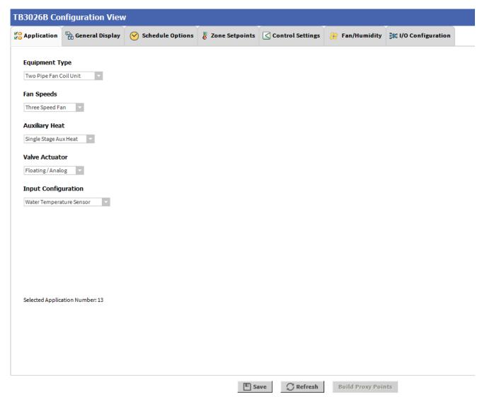
Figure 63: Two Pipe Fan Coil Unit Window
