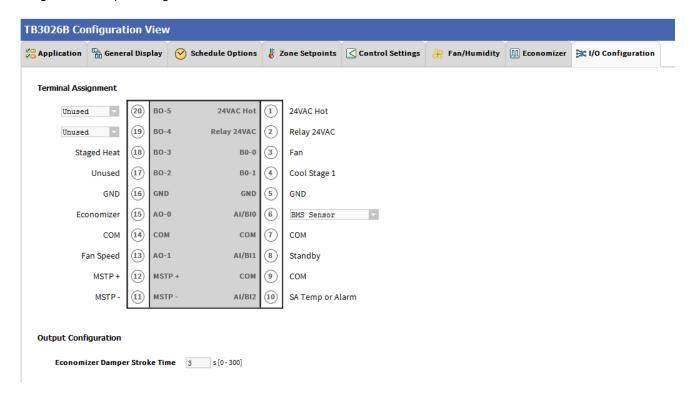
Figure 41:I/O Configurations Screen (AHU)
