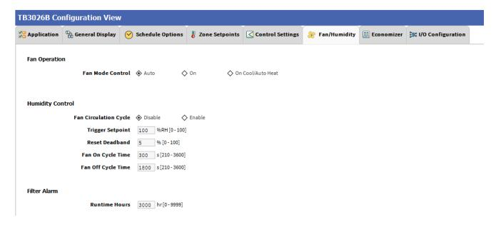
Figure 49: Fan/Humidity Screen (Air Source Heat Pump)
