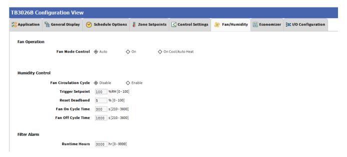
Figure 59: Fan/Humidity Screen (Water Source Heat Pump)
