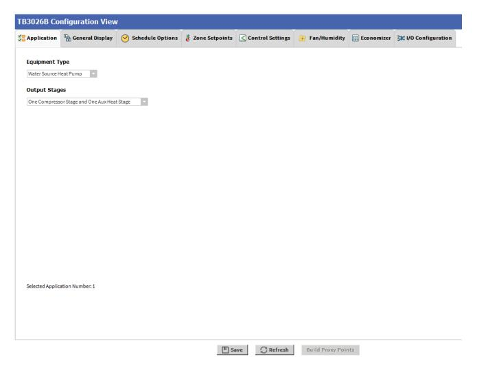
Figure 53: Water Source Heat Pump Window
