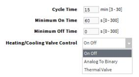
**Cycle Time:** Two-Position Valve cycle time ranges from minimum of 3 minutes, and a maximum of 30 minutes. The default value is 15 minutes.
