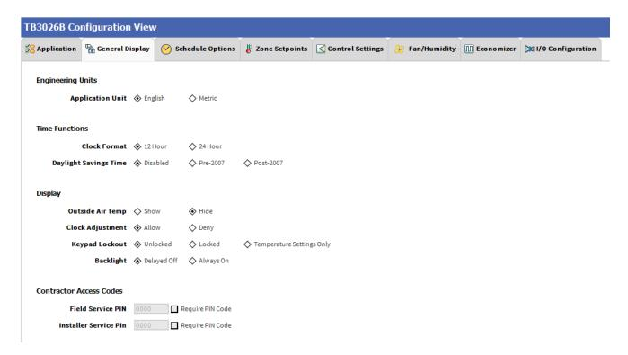
Figure 73: General Display Screen (Four Pipe Fan Coil Unit)
