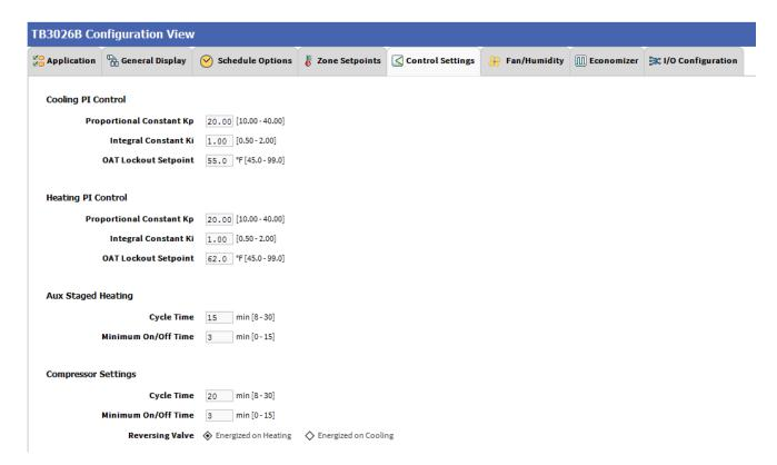
Figure 48: Control Settings Screen (Air Source Heat Pump)
