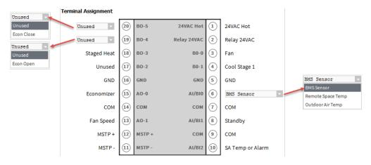
Figure 42: Terminal Assignment View (AHU)
