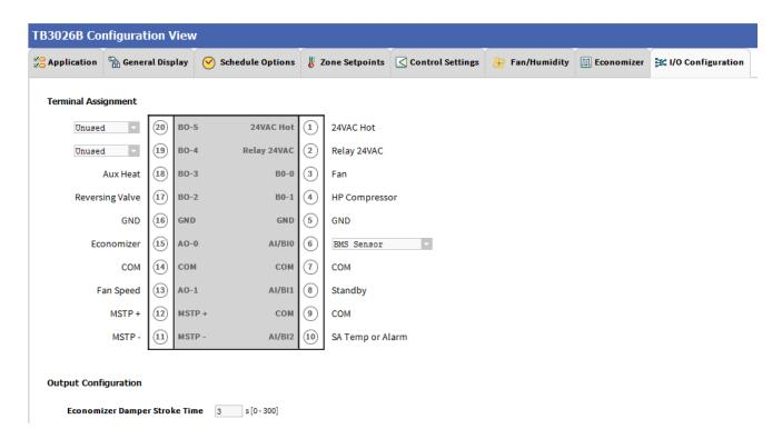
Figure 61: I/O Configurations Screen (Water Source Heat Pump)
