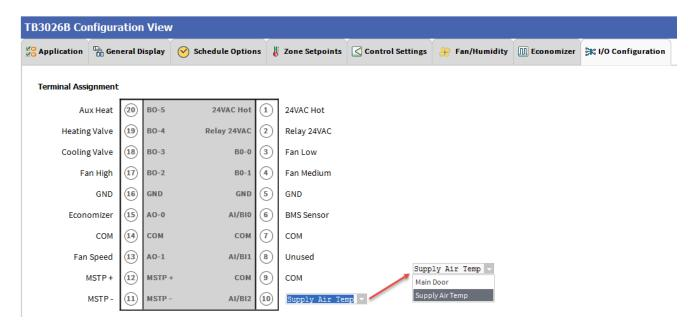
When 'Analog' valve actuator is configured, the 'Terminal Assignment' view changes as follows:
