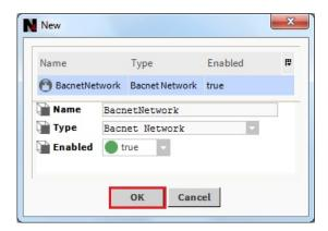
Figure 20: Adding Specification to add BACnet Network
