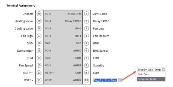
When 'Fan Speed' is selected as 'Single Speed Fan', the 'Terminal Assignment' view changes as follows:
