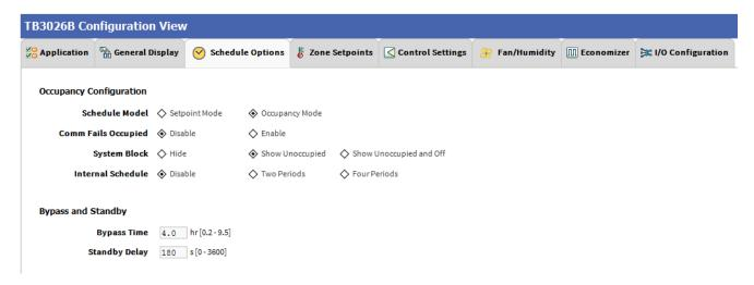
Figure 55: Schedule Options Screen (Water Source Heat Pump)
