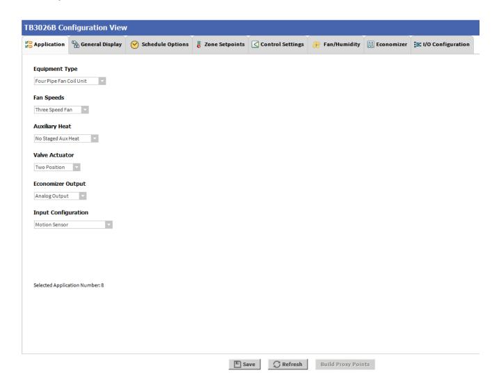
Figure 72: Four Pipe Fan Coil Unit window
