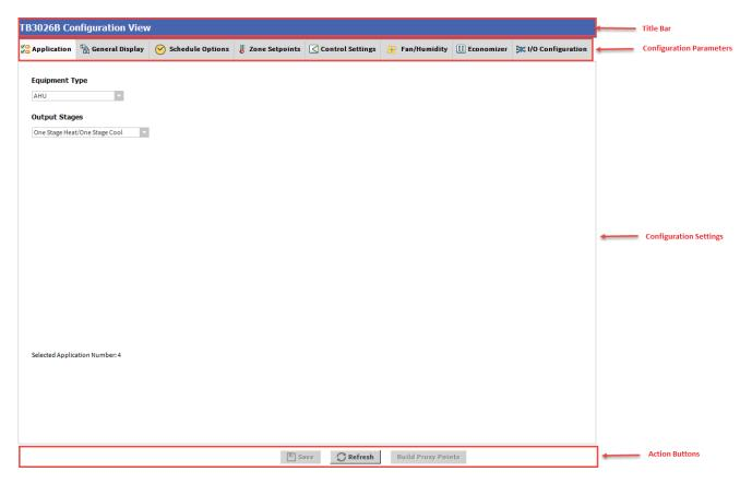
Figure 30: Field description for TB3026B Configuration Wizard Screen
