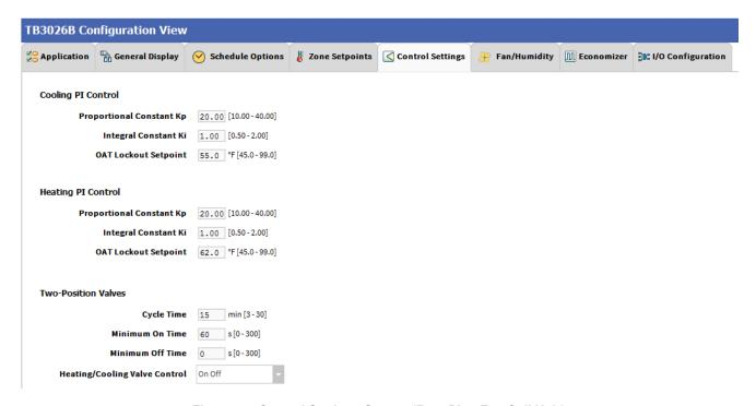
Figure 77: Control Settings Screen (Four Pipe Fan Coil Unit)
