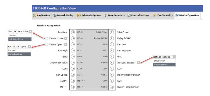
When 'No Stage Aux Heat' is configured with 'Floating/Analog' valve actuator, 'Three Speed Fan' and 'Door Switch', the 'Terminal Assignment' view changes as follows:
