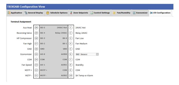
When 'Output Stage' is selected as 'One Compressor Stage/Two Aux Stages', the 'Terminal Assignment' view changes as follows:
