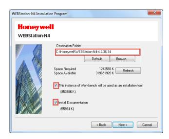
Figure 2: Installing WEBStation-N4<sup>™</sup> (selecting installation location)
