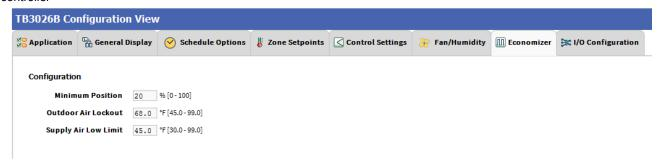
Figure 60: Economizer Screen (Water Source Heat Pump)
