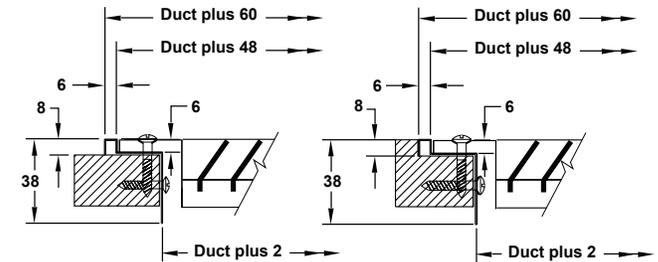
Surface Mounted Example      Recessed Mounted Example
