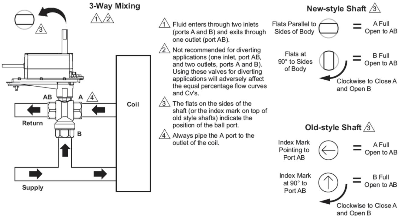
Figure 8. 3-Way Mixing Valve Assemblies Piping Diagram.
