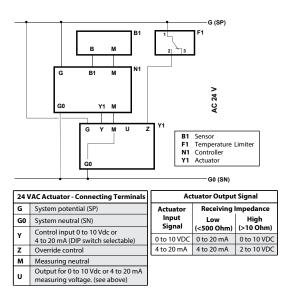
The position output signal U will switch from 0 to 10 VDC to 4 to 20 mA when a 4 to 20 mA input signal is selected and used on the Y terminal.
