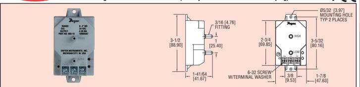
Our low cost Series 668 Differential Pressure Transmitter is capable of measuring low pressures with a  $\pm 1\%$  accuracy – ideally suited for proper building pressurization and air flow control. Transmitters can withstand up to 10 psig overpressure with no damage to the unit. Variable capacitance sensor design provides excellent sensitivity and long-term stability. Compact, lightweight design makes installation simple and easy. Units also feature reverse-polarity protection.
