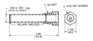
Catalog No. 34-011208-000 Low Pressure Hex Head Well (321 Stainless Steel Well & Head) Applicable Modifications Special Marking
