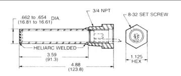
Catalog No. 34-011201-000 Hex Head Well (321 Stainless Steel Well & Head) Applicable Modifications 1 Special Marking
