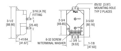
Our low cost Series 668 Differential Pressure Transmitter is capable of measuring low pressures with a ±1% accuracy ideally suited for proper building pressurization and air flow control. Transmitters can withstand up to 10 psig overpressure with no damage to the unit. Variable capacitance sensor design provides excellent sensitivity and long-term stability. Compact, lightweight design makes installation simple and easy. Units also feature reverse-polarity protection.
