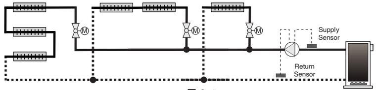
**Across Multi-Zone Radiant Manifolds with Loop Actuators**
