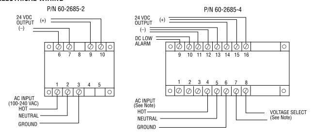
**NOTE:** For applied AC voltage of 100-120 VAC, jumper terminals 7 & 8 with shorting bar provided. For applied voltage of 200-240 VAC leave terminals 7 & 8 open.
