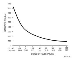
Fig. 3. C7089B sensor resistance vs. temperature performance characteristics.
